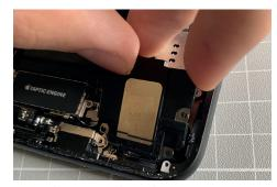
**Removing the Taptic Engine**
