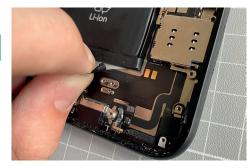
Once the adhesive strip is released, you can grab it with two fingers and pull it out from under the battery. You do not have to save the adhesive strip for reinstallation. We have packed new strips for your Fixxoo
