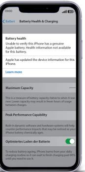
The reason is simple - from iPhone Xs/Xr onwards, the operating system checks whether the original iPhone battery is still inserted and you can ignore the error message.
