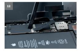
Next, disconnect the display cable plug with the tip of the spudger.
