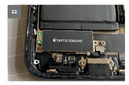
The Taptic Engine is attached with two Phillips screws on the left. Loosen them and put them aside.
