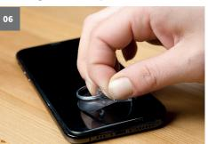
Next, remove the suction puller by pulling on the small tab at the edge. Now you can remove it from the display.
