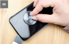
△ Be patient and gentle so as not to damage the clips. Also, be sure not to insert the lifting tool more than a few millimeters into the case, to avoid damaging the sensors at the upper end of the display.
