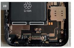
2 adhesive strips are attached to the lower and upper edge (not shown) of the battery. These hold the battery firmly in position.
