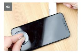
Starting from the lower-left corner, slide the lifting tool up the left side of the frame (to the position of the mute button), to separate the glue seal holding the display and frame together.
