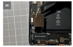
The SIM card reader is now free and can be lifted out of the housing with the tweezers.
