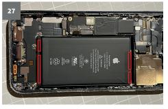
There are two adhesive strips on each side of the battery, which you peel off and sl wly pull out from under the battery. Start at the bottom end.
