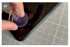
Now remove the suction cup by pulling on the small knob. You can now remove it from the display.
