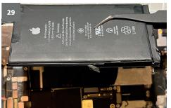
Once you have removed all the adhesive strips, you can carefully remove the battery.
