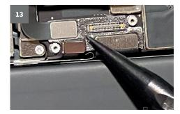
Underneath, the path to the touchscreen cable connector is cleared. This is also removed.
