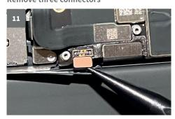
• Remove the battery plug with the tip of the spudger.
