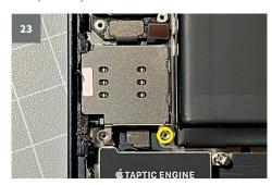
This will reveal another screw, this time a spacer screw (standoff). Loosen this as well.
