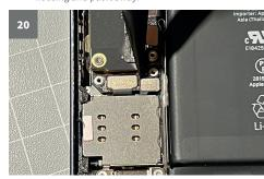
Underneath is the plug of the SIM card reader, which you lever out with the spudger.
