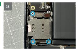
Three triwing screws secure the sim card reader. Remove these.
