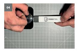
① Do not push the lifting tool too deep into the iPhone, otherwise you may damage internal components.
