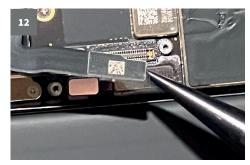
The display connector, which you remove next, is located above the removed battery connector.
