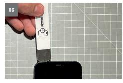
Cut through the remaining adhesive on the upper frame by pushing the lifting tool to the left.
