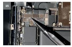
Now the connector for the front sensors is still free, which you disconnect in the same way.
