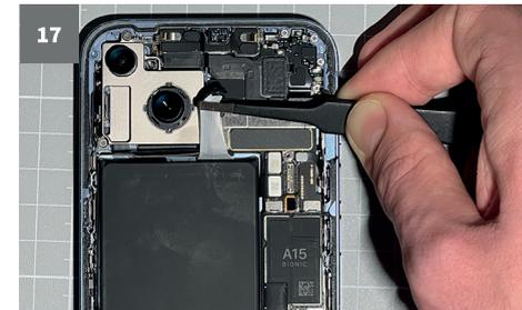
⚠ If one of the adhesive strips tears: Please do not use force. The battery must not be squeezed or bent. A little solvent dripped under the battery or heating with a hair-dryer often helps.
