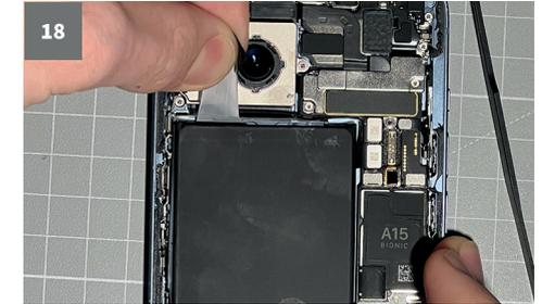
⚠ Work carefully so that you do not touch the sensor modules at the top edge. Otherwise they could be destroyed.
