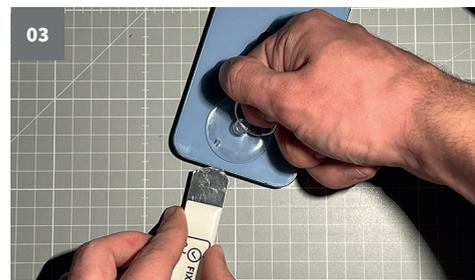
**Separate the glue seal between the cover glass and the frame.**
