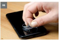
Next, remove the suction puller by pulling on the small tab at the edge. Now you can remove it from the display.
