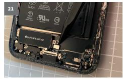
Next, loosen the plug of the taptic enginge with the spudger.
