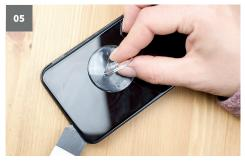
Completely separate the rest of the glue at the upper end of the frame by sliding the lifting tool to the left.
