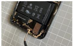
Now remove the screw that secures the cover of the speaker connector and then lift the cover out of the housing with the tweezers.
