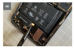
Use the spudger to remove the speaker plug from the housing.
