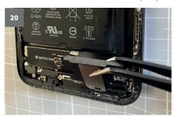
Then you can lift the speaker out of the housing with the tweezers.
