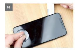
Starting from the lower-left corner, slide the lifting tool up the left side of the frame (to the position of the mute button), to separate the glue seal holding the display and frame together.
