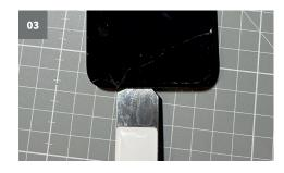
Starting from the lower-left corner, slide the lifting tool up the left side of the frame (to the position of the mute button), to separate the glue seal holding the display and frame together.
