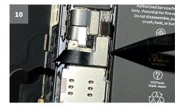
The display connector (with a QR code print), which you remove next, is located below the removed battery connector.
