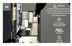
· Remove the battery plug with the tip of the spudger.
