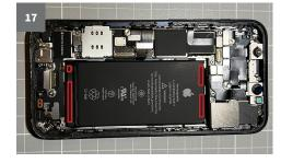
There are two adhesive strips on each side of the battery, which you peel off and sl wly pull out from under the battery. Start at the bottom end.
