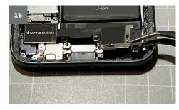
• The unit can now be easily removed with the tweezers.
