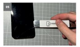
Completely separate the rest of the glue at the upper end of the frame by sliding the lifting tool to the left.
