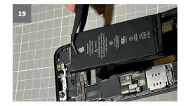
Once you have removed all the adhesive strips, you can carefully remove the battery.
