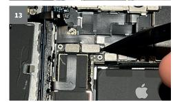
⚠ Important: The ribbon cable must not be stretched in order not to damage it.
